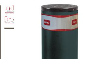
Anti-terrorist hydraulic bollard with incorporated hydraulic control unit. Suitable for protecting sensitive sites, thanks to the special "SD" version, which keeps the shaft raised in case of a power failure and with public installations where, in the standard version, the shaft lowers automatically with no power.
